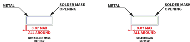
Figure 9.2 SOP16(300mil)/SOW16 Package Board Layout Example
