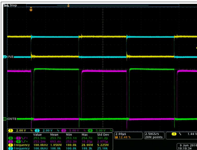
Figure 41. Bench Test Waveform for INA/B and OUTA/B
