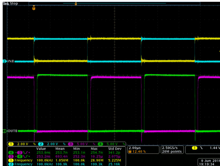
Figure 8-5. Bench Test Waveform for INA/B and OUTA/B
